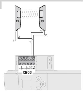
A connected photocell is automatically detected by the controller as soon as the power supply is connected. The photocell can be retrospectively reprogrammed.
