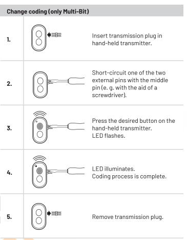
After recoding the hand-held transmitter, the drive system must also be reprogrammed to the new coding.
