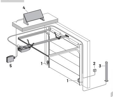
The gate system is an example and may vary depending on gate type and equipment. The system shown consists of the following components:
