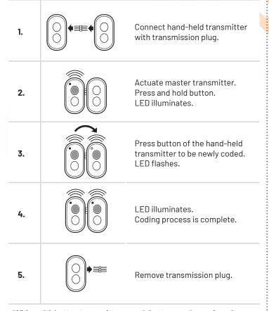
With multi-button transmitters, each button can be assigned a separate function.
