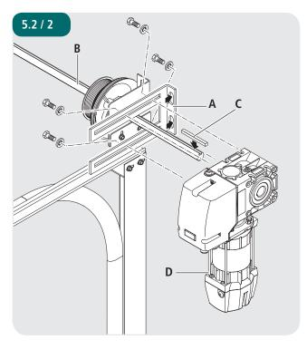
Fit the torque support bracket/console (A).
