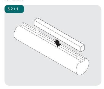
Check whether the feather key is suitable for the spring shaft on site.
