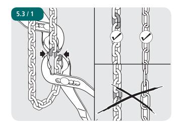
Join the ends of the emergency hand chain together with the chain connecting link.
